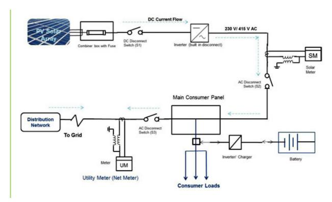
The utility meter (Net-meter) has to be bi-directional meter to register both import grid electricity amount as well as export solar electricity amount.
